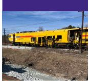
The tamping machine at Høje Taastrup Station contributing to a significant upgrade of Denmark's main traffic hubs. The contract covers track renewal including the replacement of 19 points.
