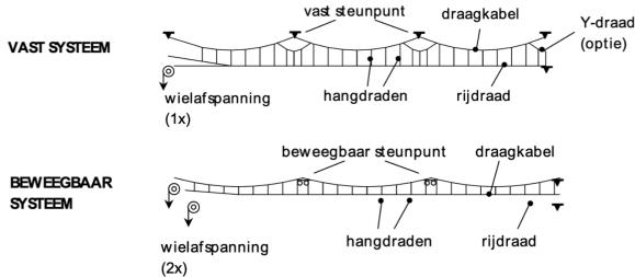
Visualization of an overhead line. In the Netherlands, there is both a fixed system and movable overhead wires. For the chain analysis, it is not important which system is used. It only concerns the contact wires that are the same in both systems.
